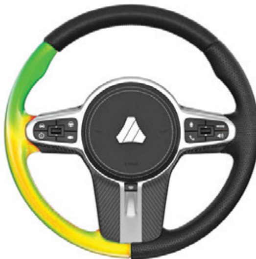
Simulation-driven design of a steering wheel with polyurethane foam manufacturing analysis
