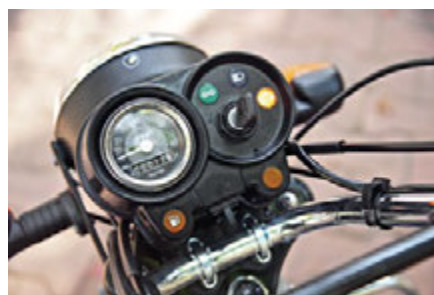
ABOVE: Intelligent console has a fuel reserve light, too
